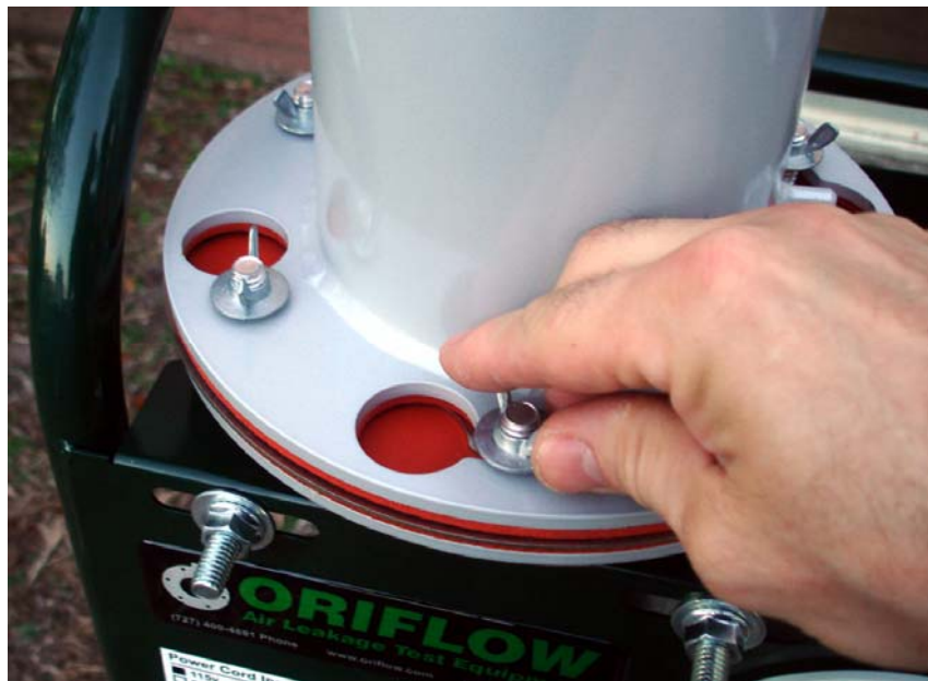
Figure 4 – Tighten Wing Nuts after Rotation
