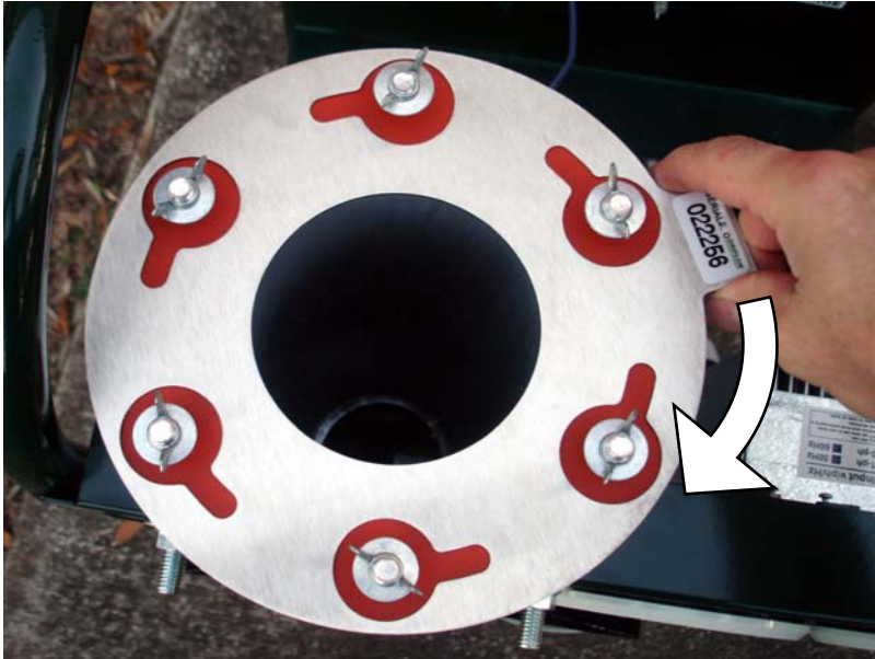
Figure 1 – Install Orifice Plate and then Rotate Clockwise
