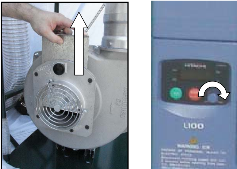
Figure 15 – Obtaining System Test Pressure
