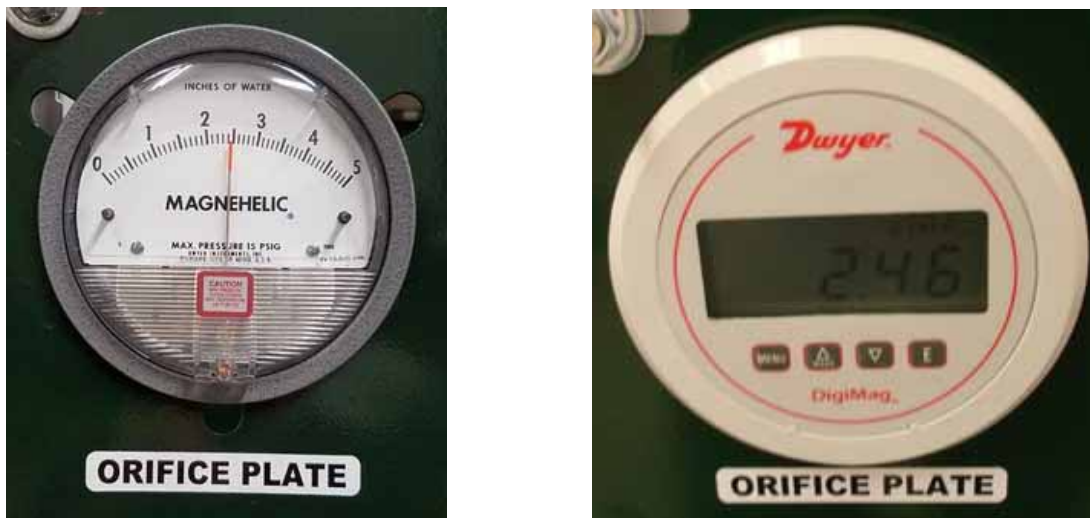
Figure 14 –ORIFICE PLATE Gauge Reading (analog on left, digital on right)
