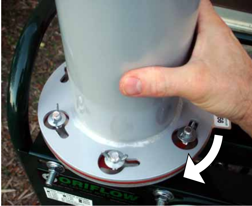
Figure 3 – Install Upper Tube Section and Rotate Clockwise
