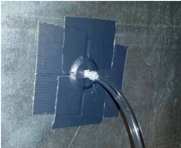
Figure 7 – Connection to Duct System using Static Pressure Tap
