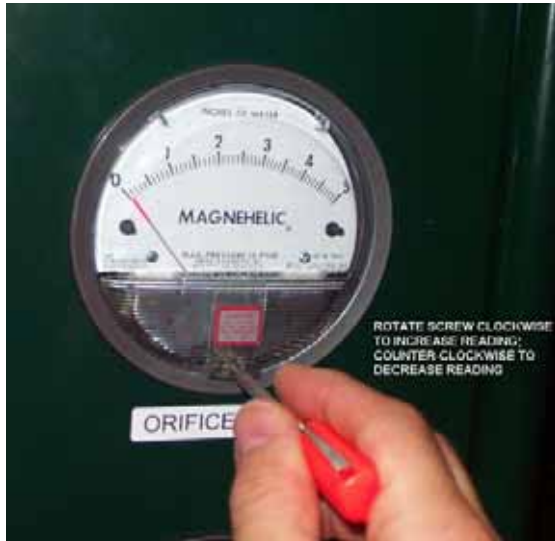
Figure 10 – Zeroing Analog Gauges
