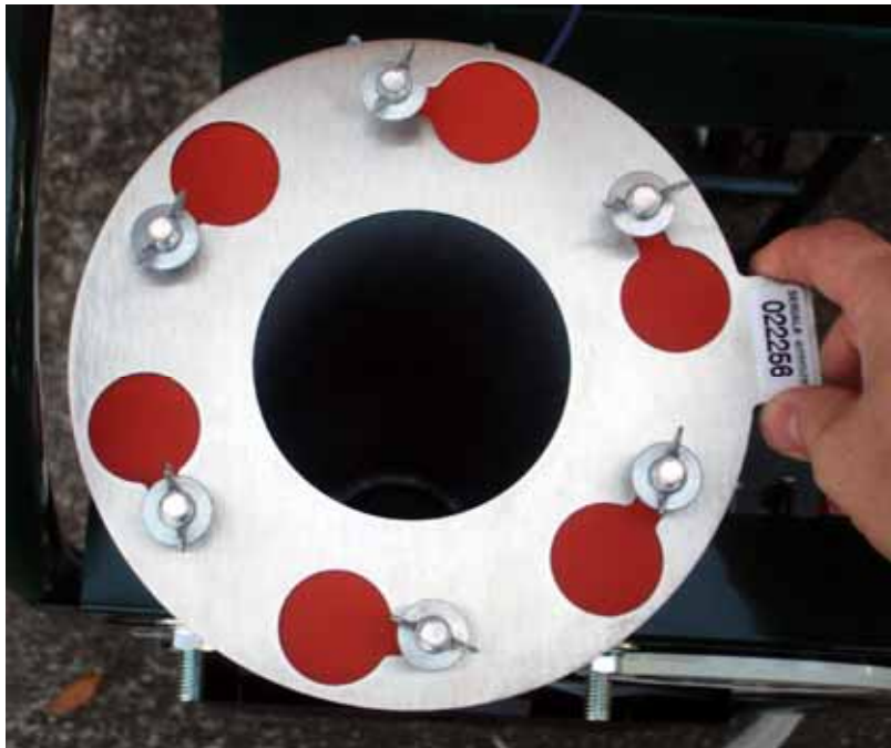
Figure 2 – Rotate Orifice Plate Clockwise until it Locks in Place
