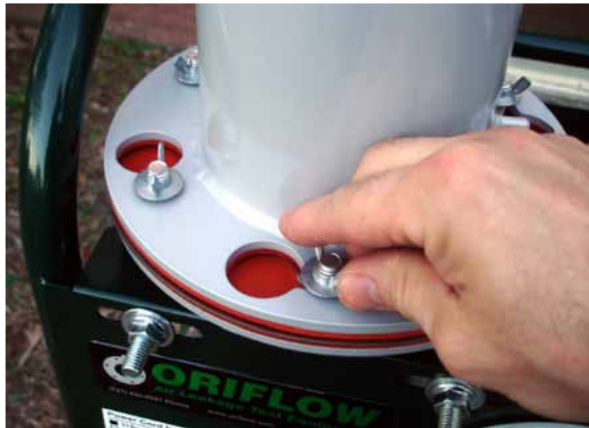
Figure 4 – Tighten Wing Nuts after Rotation
