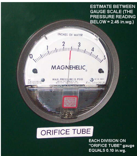
Figure 15 –ORIFICE PLATE Gauge Reading (analog on left, digital on right)
