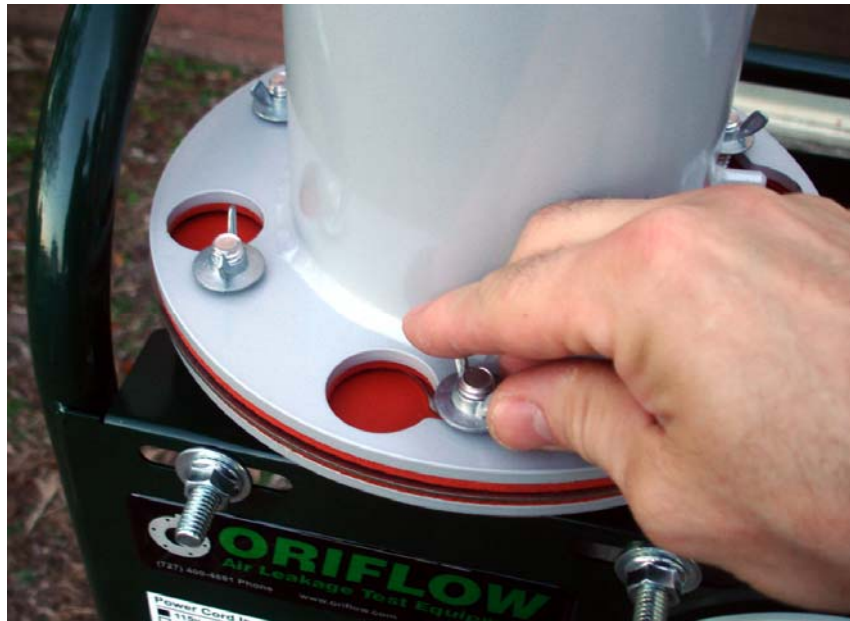
Figure 4 – Tighten Wing Nuts after Rotation
