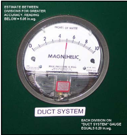
Figure 14 – Duct System Gauge Reading (analog on left, digital on right)
