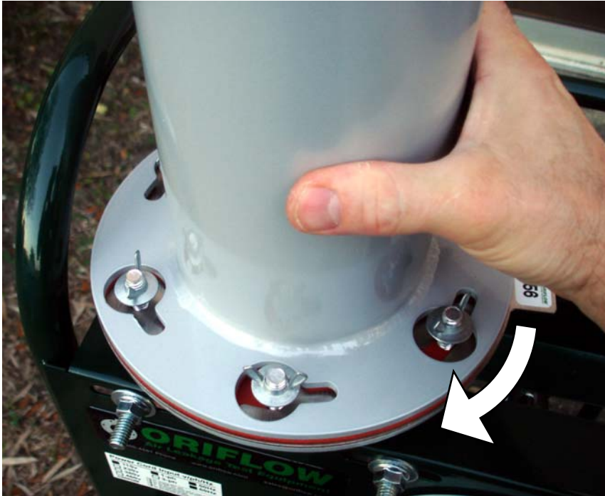
Figure 3 – Install Upper Tube Section and Rotate Clockwise
