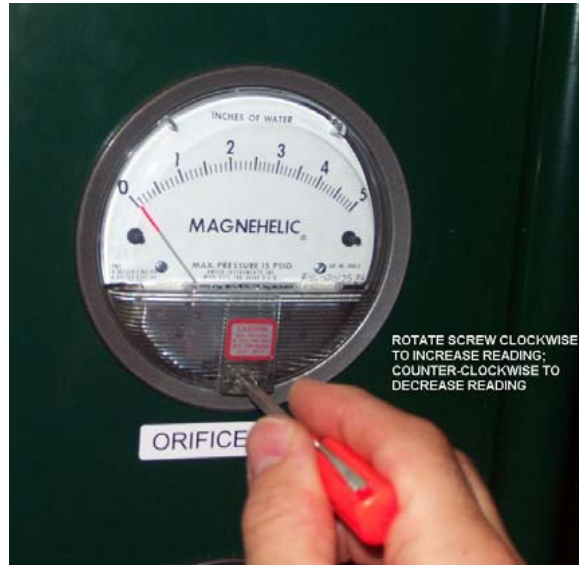
Figure 11 – Zeroing Analog Gauges
