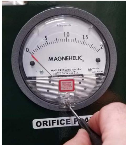
**Figure 11** – Zeroing Analog Gauges
