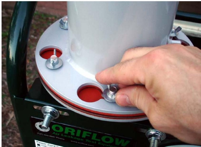
**Figure 4** – Tighten Wing Nuts after Rotation
