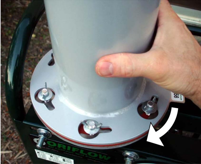
**Figure 3** – Install Upper Tube Section and Rotate Clockwise
