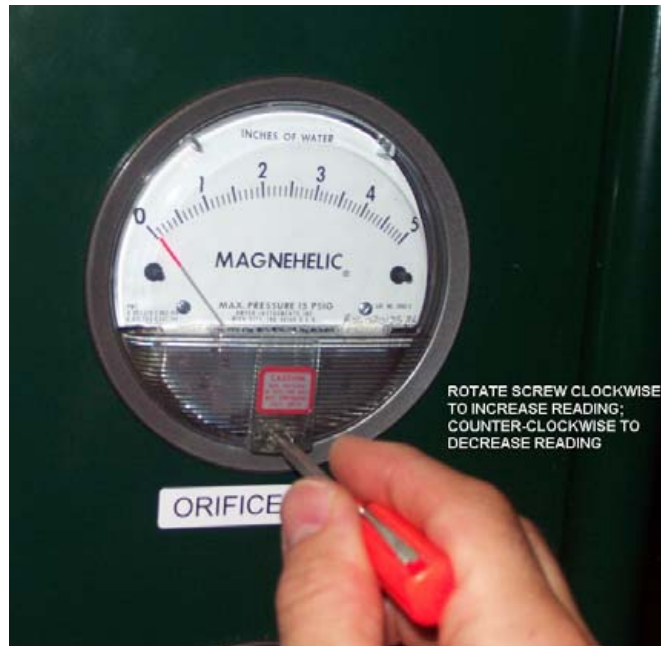
Figure 10 – Zeroing Analog Gauges (zero BOTH gauges before testing)
