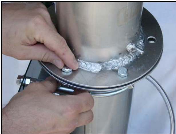
Figure 3 – Bolting Flange (hand tighten snugly)
