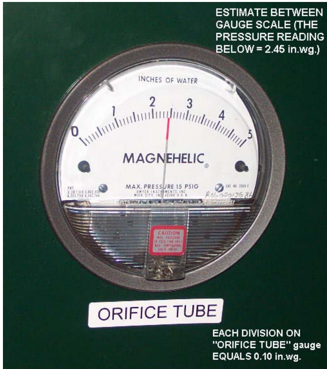
Figure 15 –ORIFICE TUBE reading
