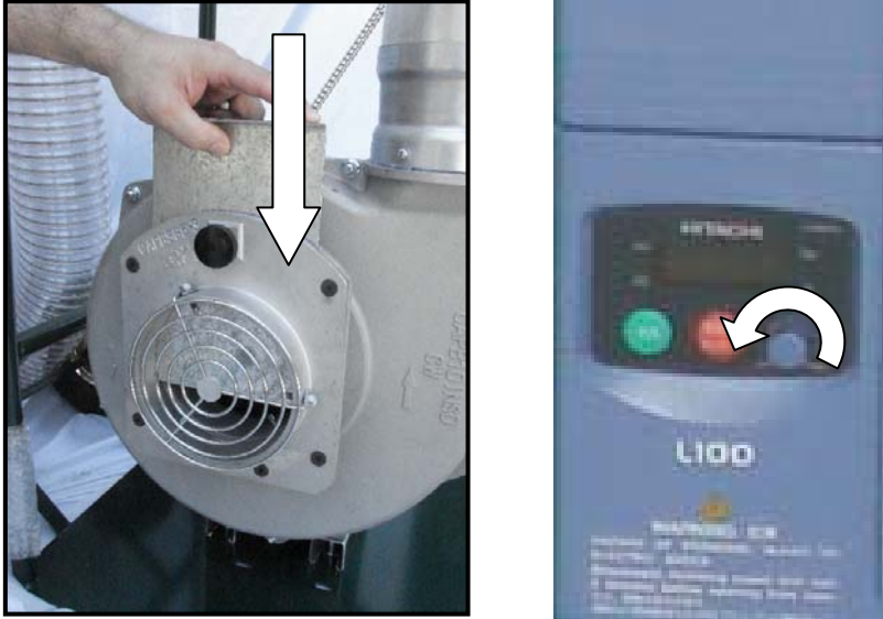
Figure 12 – Avoid Over-Pressurizing by Minimizing Air Delivery upon Startup
